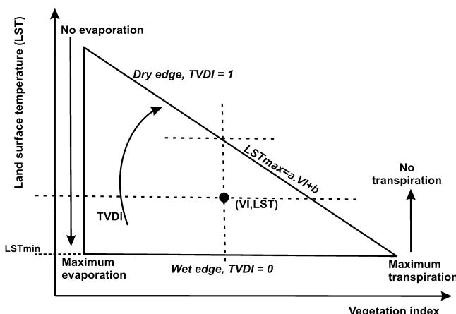
**Fig. 1.** Conceptual diagram of LST-vegetation index scatterplot for defining Temperature Vegetation Dryness Index (TVDI). The position of a given pixel (VI, LST) is determined mainly by soil moisture availability.
