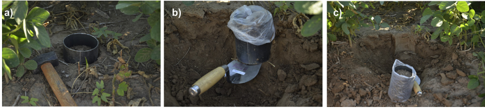
Fig. 1. Sampling of undisturbed soil (10 cm depth) using a metal cylinder.
