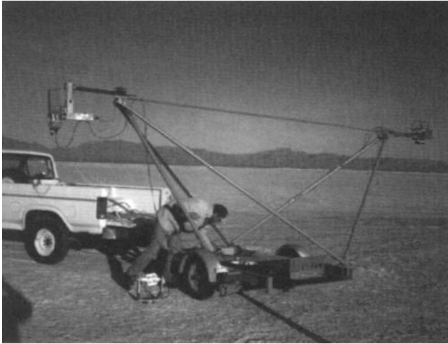
Figure 7.11 The reflectomobile used by Slater et al. (1987) in calibration of satellite sensors. The radiometers were calibrated in the field with reflectance standards and then driven over a study site to generate mean reflectance over a large, approximately uniform surface.
