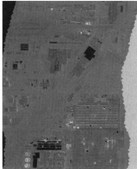
Figure 6.5 Tangent error effects. The diagonal roads in the thermal infrared line scanner image should be straight, and the tanks in the lower left roughly circular. (b) Original image and (c) image after tangent correction.
