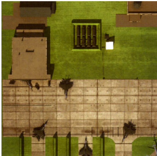
Plate 14.16 A true-color synthetic scene produced by DIRSIG showing texture effects. Note this is the same scene shown in the model board in Figure 14.1.
