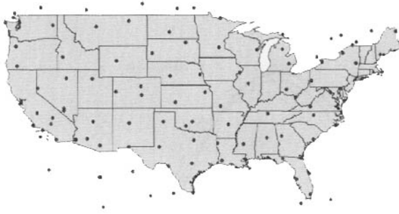
Figure 7.19 Map of radiosonde stations. Balloons are released twice daily at 12:00 and 24:00 Greenwich.
