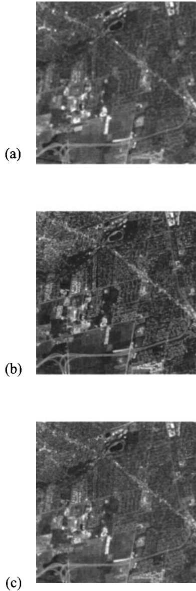
Figure 12.18 Fusion of multispectral TM data (a) with geometrically registered and resampled SPOT data (b) to yield the fused product (c). See color plate 12.18.
