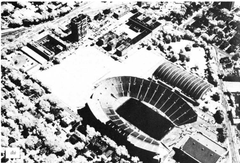
Figure 2.24 Simultaneous oblique aerial photographs showing the effect of filtration on discrimination of ground objects. On panchromatic film (a) natural grass and artificial turf have a similar tone. When scene energy is filtered such that only wavelengths longer than 0.7 \mu\text{m} are incident on black and white IR film (b), the natural grass has a very light tone and the artificial turf a very dark tone.
