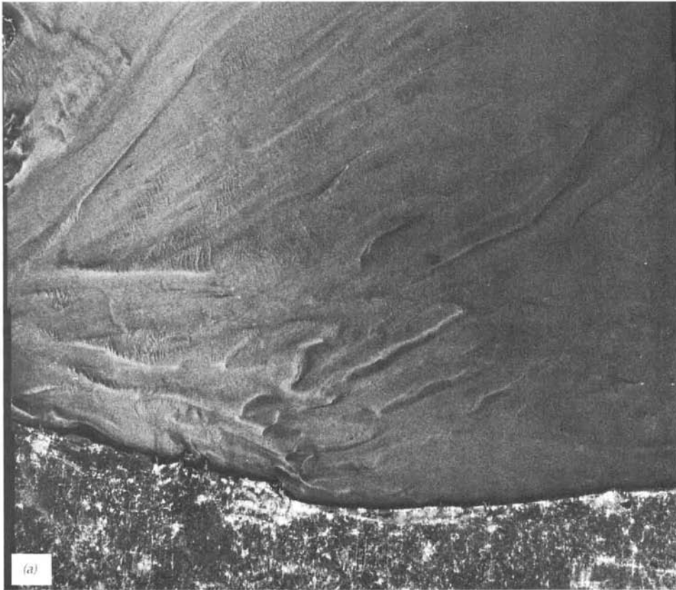
Figure 8.33 English Channel near the Strait of Dover: (a) Seasat SAR image, L band, midsummer; (b) map showing ocean bottom contours in meters. (Courtesy NASA/JPL/Caltech.)
