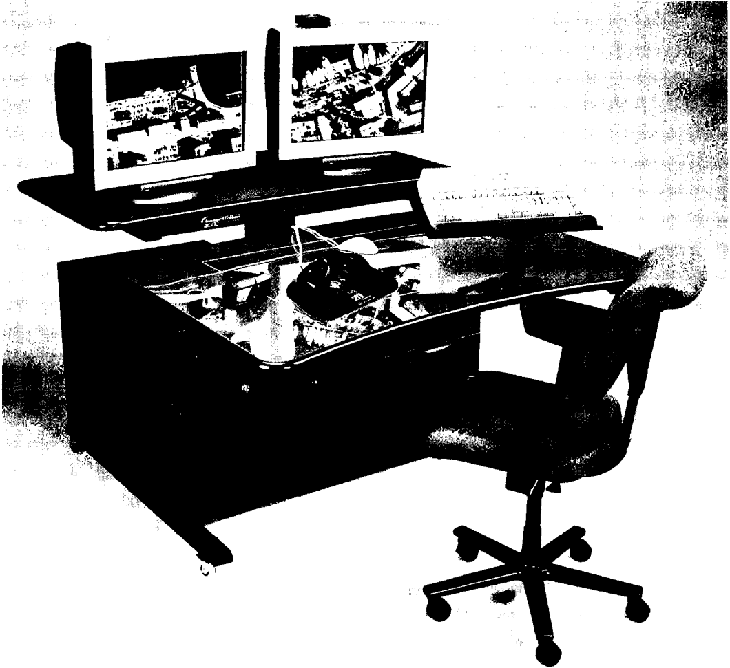
Figure 3.29 Z/I Imaging ImageStation 2002 digital photogrammetric workstation (shown with optional dual monitors). System employs an infrared emitter (on top of right monitor) and liquid-crystal glasses (left side of digitizing table) for stereoscopic viewing. (Courtesy Z/I Imaging Corporation.)
