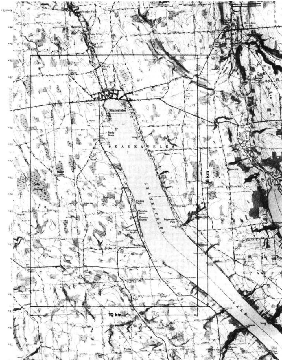
Figure 3.34 A 10 × 16-km study area over which photographic coverage is to be obtained.
