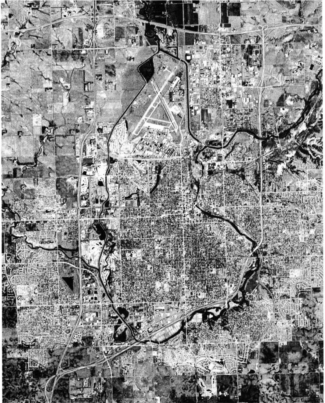
Figure 6.16 The first image acquired by the Landsat-7 ETM+. Panchromatic band (15 m resolution), Sioux Falls, SD, April 18, 1999. Scale 1: 88,000. (Courtesy EROS Data Center.)
