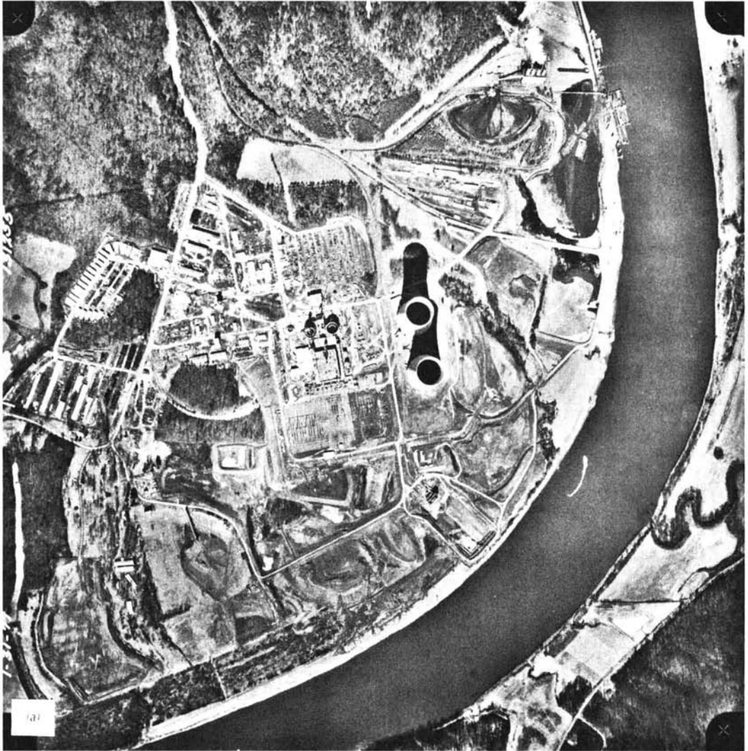
Figure 3.12 Vertical photographs of the Watts Bar Nuclear Power Plant Site, near Kingston, TN. In (a) the two plant cooling towers appear near the principal point and exhibit only slight relief displacement. The towers manifest severe relief displacement in (b). (Courtesy Mapping Services Branch, Tennessee Valley Authority.)
