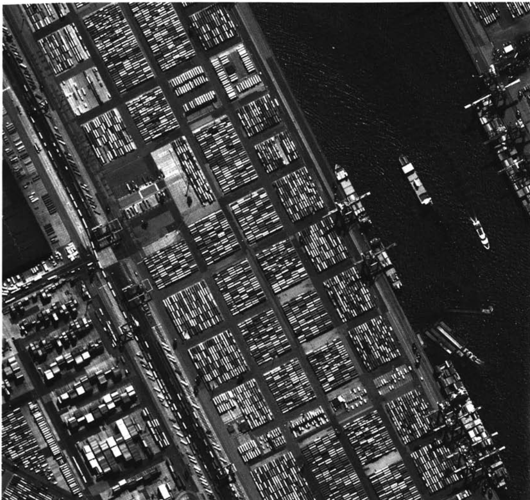
Plate 20 High resolution satellite imagery from QuickBird showing a portion of the Port of Hamburg, Germany. The image is the result of applying pan-sharpening techniques to a true-color composite of multispectral bands 1, 2, and 3 shown as blue, green, and red, respectively, and has an effective resolution of 61 cm. (Courtesy Digital-Globe.) (For major discussion, see Section 6.15.)
