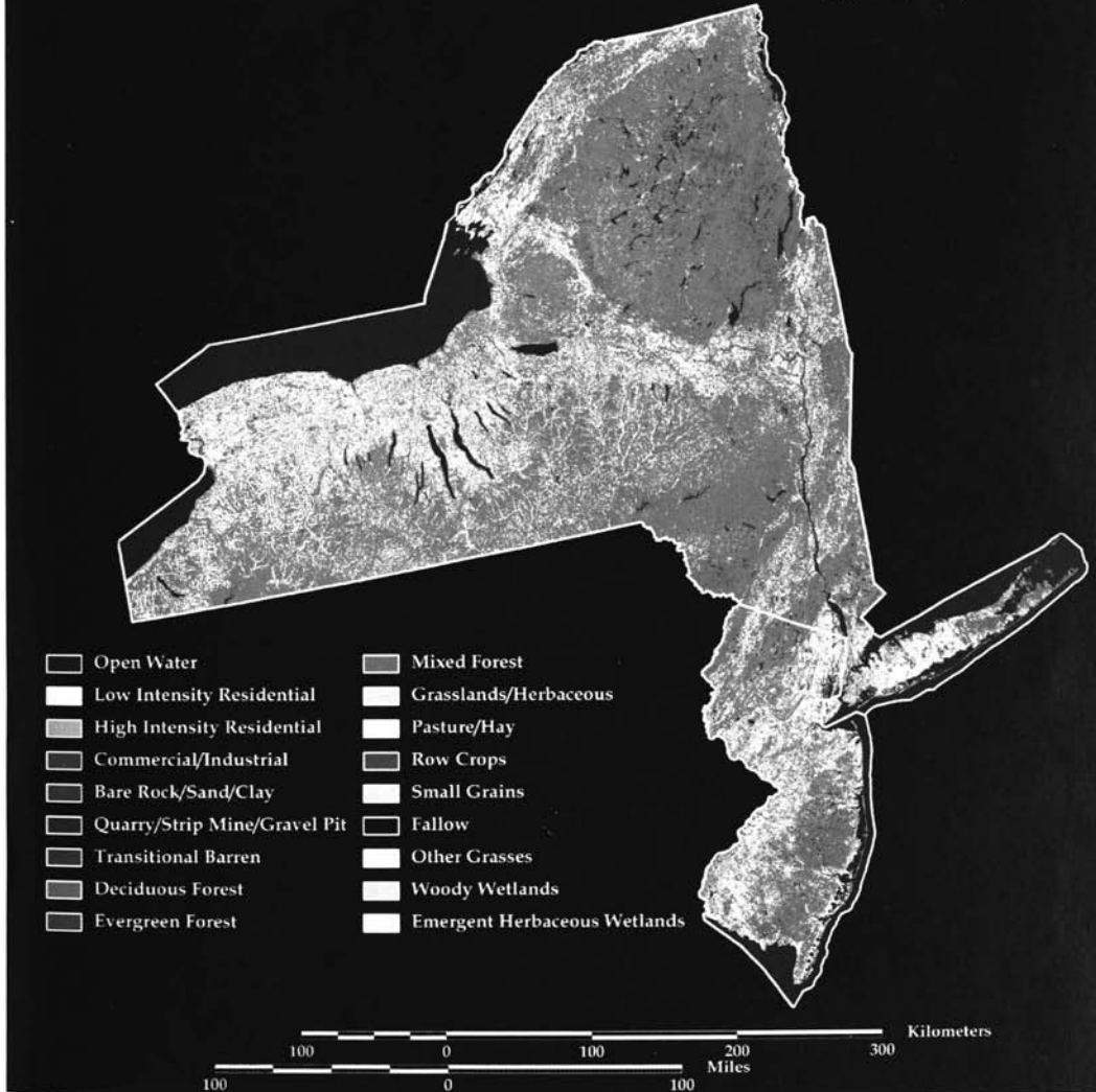
Plate 30 New York and New Jersey land cover derived from Landsat Thematic Mapper data. (Courtesy US EROS Data Center.) (For major discussion, see Section 7.14.)
