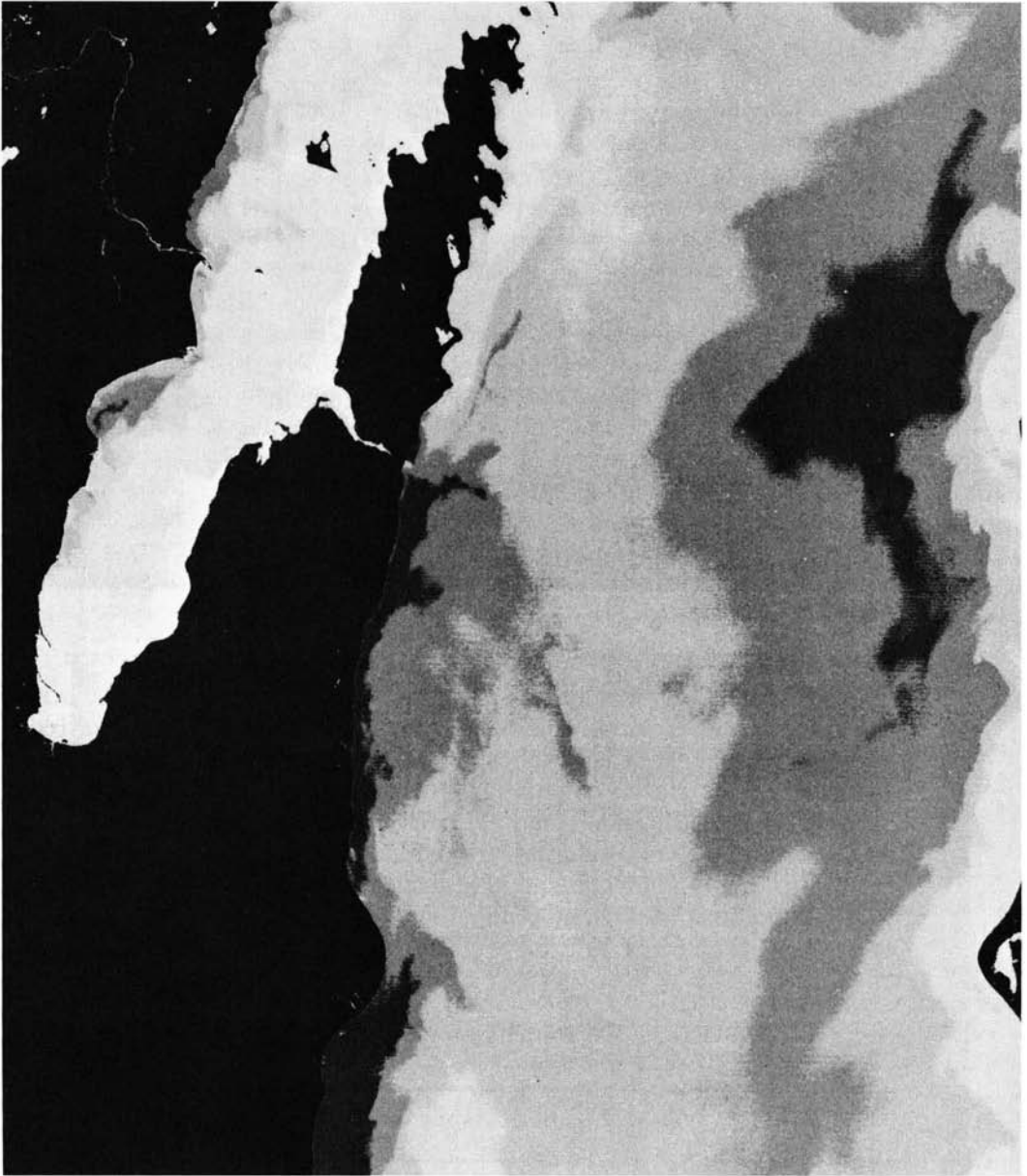
Figure 6.18 Landsat TM band 6 (thermal IR) image, Green Bay and Lake Michigan, Wisconsin–Michigan, mid-July. Scale 1: 225,000.
