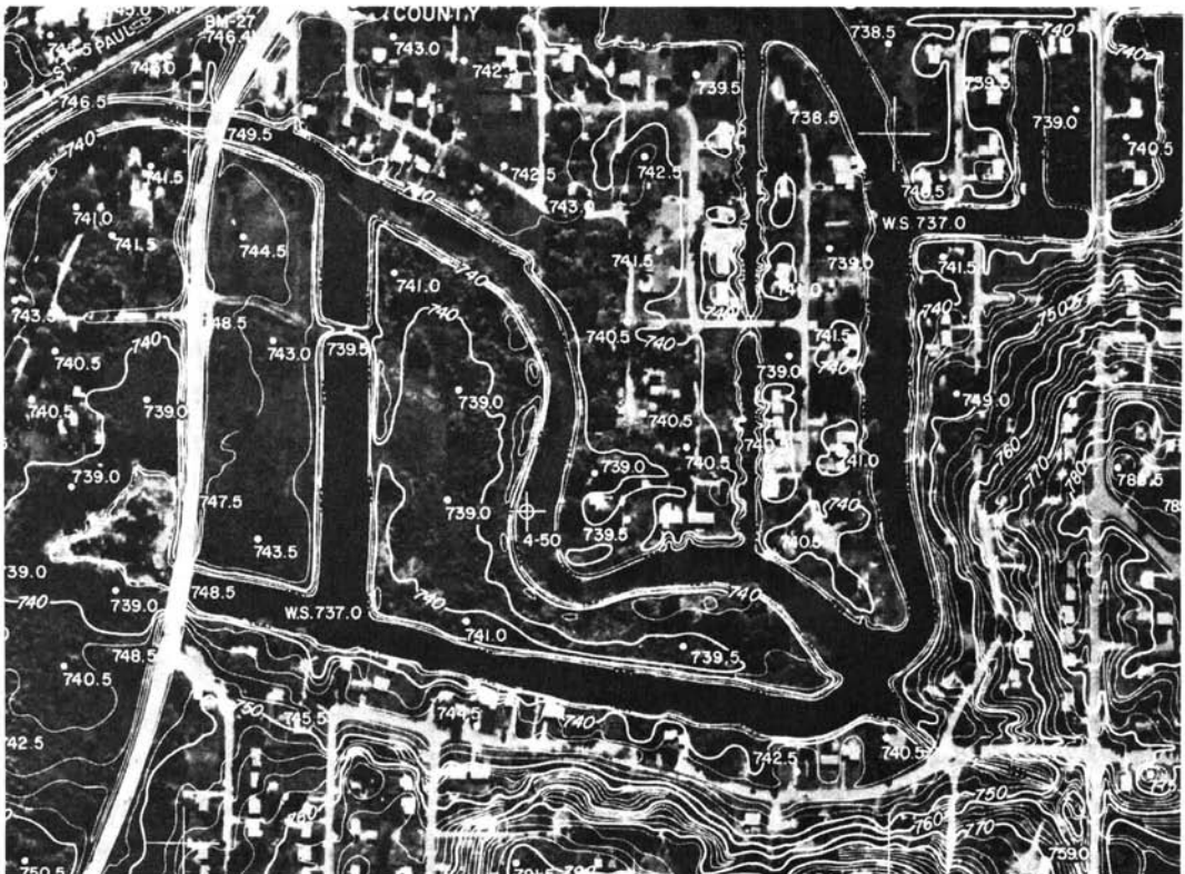
Figure 3.27 Portion of a 1:4800 topographic orthophotomap. Photography taken over the Fox Chain of Lakes, IL. (Courtesy Alster and Associates, Inc.)
