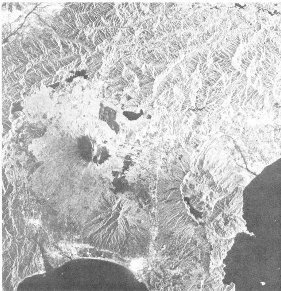
Figure 8.45 JERS-1 radar image showing Mt. Fuji and vicinity, Japan. Scale 1:450,000. (NASDA, 1992. Courtesy Remote Sensing Technology Center of Japan.)
