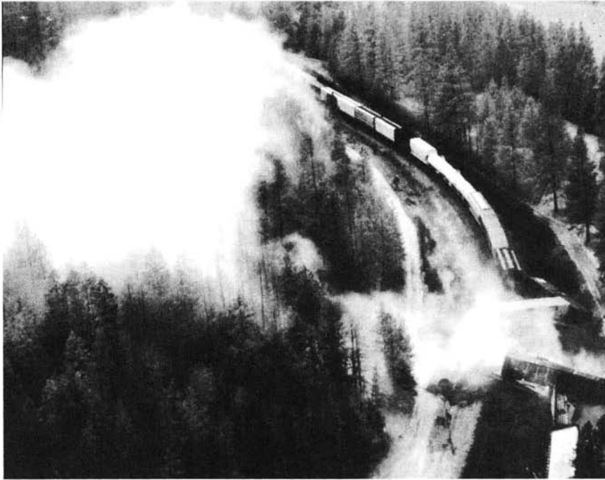
Figure 4.42 Low altitude, oblique aerial photograph of chlorine spill resulting from train derailment near Alberton, MT. (Courtesy RMP Systems.)
