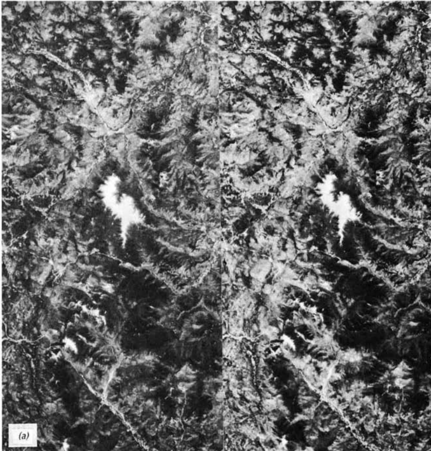
Figure 3.3 Large Format Camera stereopairs, Mt. Washington and vicinity, New Hampshire, April 4, 1985; scale 1:800,000 (1.5 times enlargement from original image scale); (a) 0.30 base-height ratio; (b) 1.2 base-height ratio. (Courtesy NASA and ITEK Optical Systems.)
