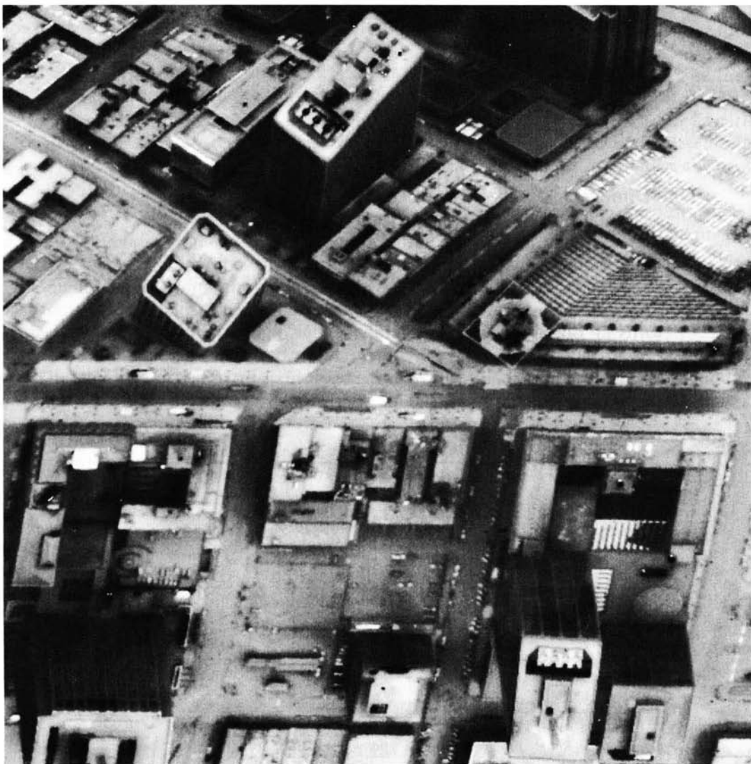
Figure 5.31 Across-track thermal scanner image illustrating one-dimensional relief displacement, San Francisco, CA, predawn, 1500-m flying height, 1 mrad IFOV. (Courtesy NASA.)
