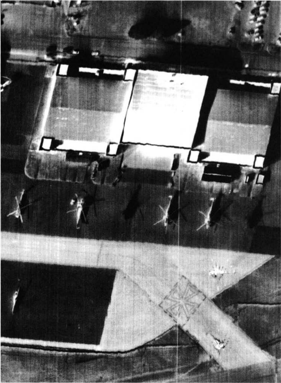
Figure 5.20 Daytime thermal image, Quantico, VA, 0.25 mrad IFOV. (Courtesy RECON/OPTICAL, Inc.)
