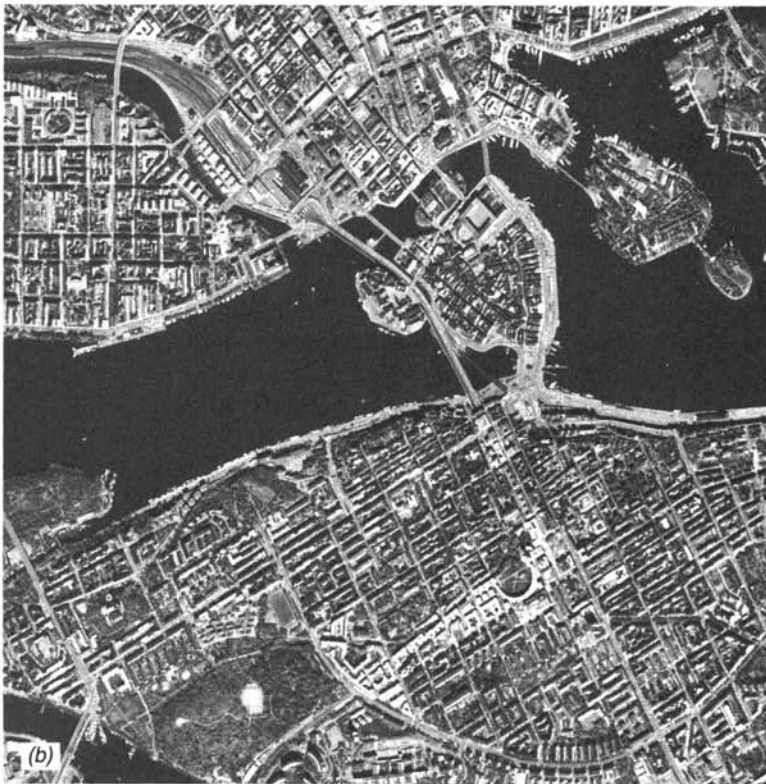
Figure 6.30 SPOT-5 HRG imagery of Stockholm, Sweden, May, 2002: (a) Band 2, 10 m resolution (red); (b) panchromatic band, 2.5 m resolution. (Courtesy CNES and SPOT Image, Inc.)
