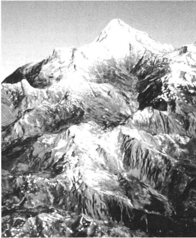
Figure 6.28 Perspective view of the Albertville area in the French Alps, generated entirely from SPOT data, on successive days in late July. (Produced by ISTAR. Copyright © 1993 CNES. Provided by SPOT Image Corp.)
