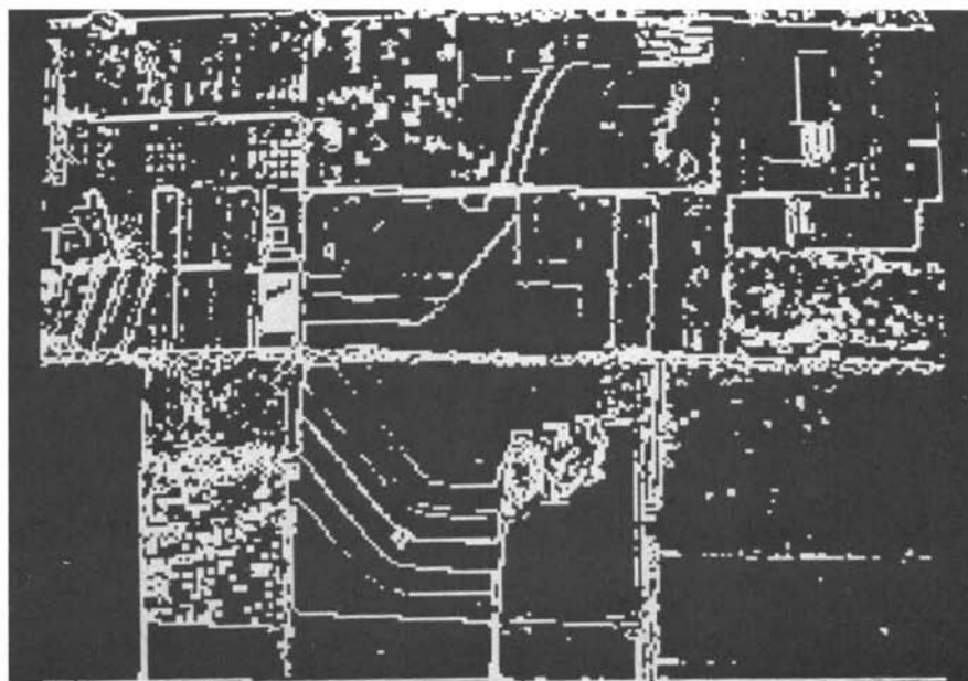
Figure 7.21 Edge enhancement through cross-diagonal first differencing.
