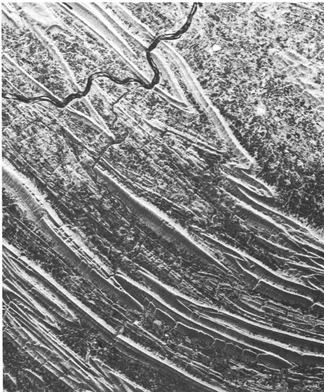
Figure 8.3 Seasat SLR image of Appalachian Mountains of Pennsylvania, L band, midsummer. Scale 1 : 575,000. (Courtesy NASA/JPL/Caltech.)
