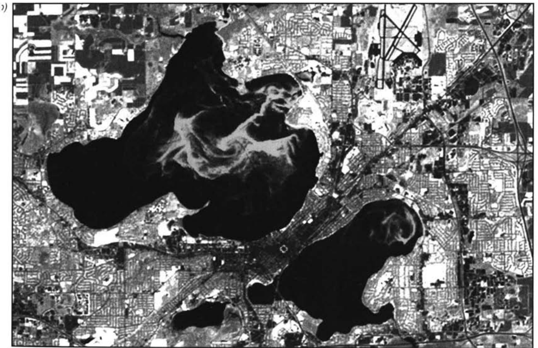
Plate 31 Multitemporal NDVI data merging. (a) Using multitemporal data as an aid in mapping invasive plant species, in this case reed canary grass (shown in red to pink tones) in wetlands. This color composite results from the merger of NDVI values derived from Landsat-7 ETM+ images of southern Wisconsin acquired on March 7 (blue), April 24 (green), and October 15 (red), respectively. Scale 1:120,000. (b) Monitoring algal blooms in portions of the two northernmost lakes shown. NDVI values derived from Landsat-7 ETM+ images acquired on April 24 (blue), October 31 (green), and October 15 (red), respectively. Scale 1:130,000. (For major discussion, see Section 7.17.)
