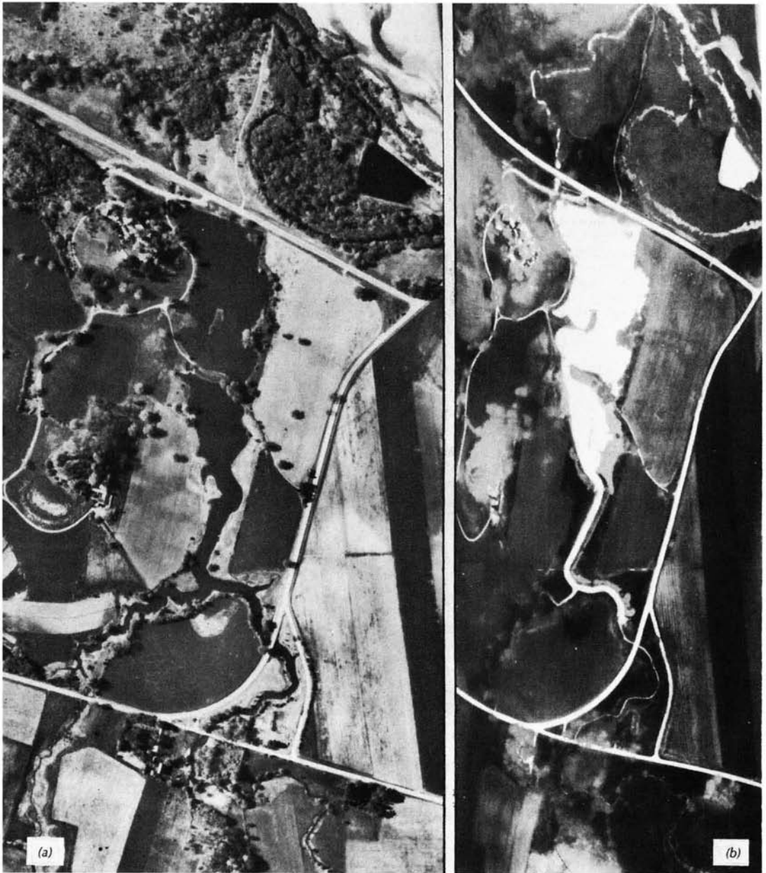
Figure 5.26 Comparison of aerial photograph and across-track thermal scanner image illustrating tangential distortion, Iowa County, WI: (a) panchromatic aerial photograph, 3000-m flying height; (b) nonrectified thermal image, 6:00 A.M., 300-m flying height. [(a) Courtesy USDA-ASCS. (b) Courtesy National Center for Atmospheric Research.]
