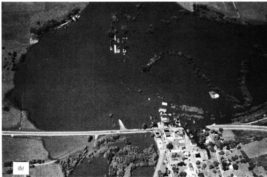
Figure 4.24 Black and white copies of panchromatic and color infrared aerial photographs showing flooding and its aftereffects, Pecatonica River near Gratiot, WI: (a) USDA–ASCS panchromatic photograph. Scale 1: 9000. (b) Oblique color infrared photograph, June 30. (c) Oblique color infrared photograph, July 22. (d) Oblique color infrared photograph, August 11. The flying height for photos (b) to (d) was 1100 m.
