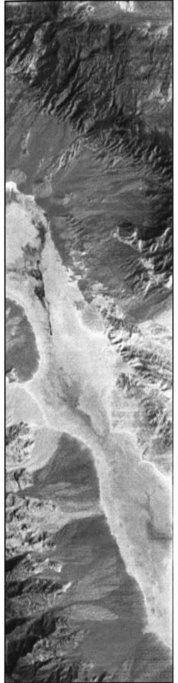
Plate 27 ASTER data, Death Valley, CA, early March. (a) VNIR (visible and near-IR) bands 1, 2, and 3 displayed as blue, green, and red, respectively. (b) SWIR (mid-IR) bands 5, 7, and 9 displayed as blue, green, and red, respectively. (c) TIR (thermal IR) bands 10, 12, and 13 displayed as blue, green, and red, respectively. Scale 1:350,000. (For major discussion, see Section 6.18.)
