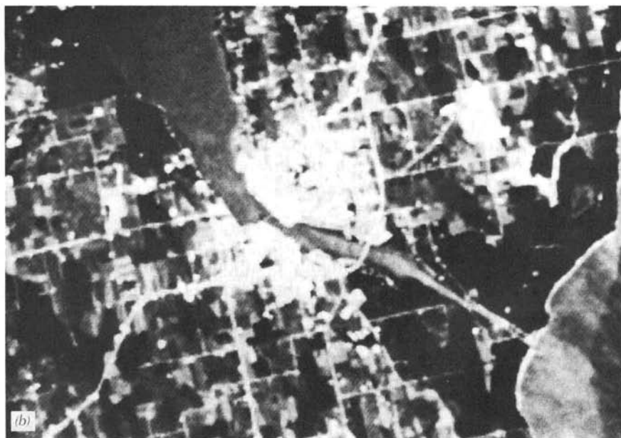
Figure 7.18 Frequency components of an image resulting from varying the kernel used for convolution: (a) original image; (b–d) successively lower frequency enhancements.
