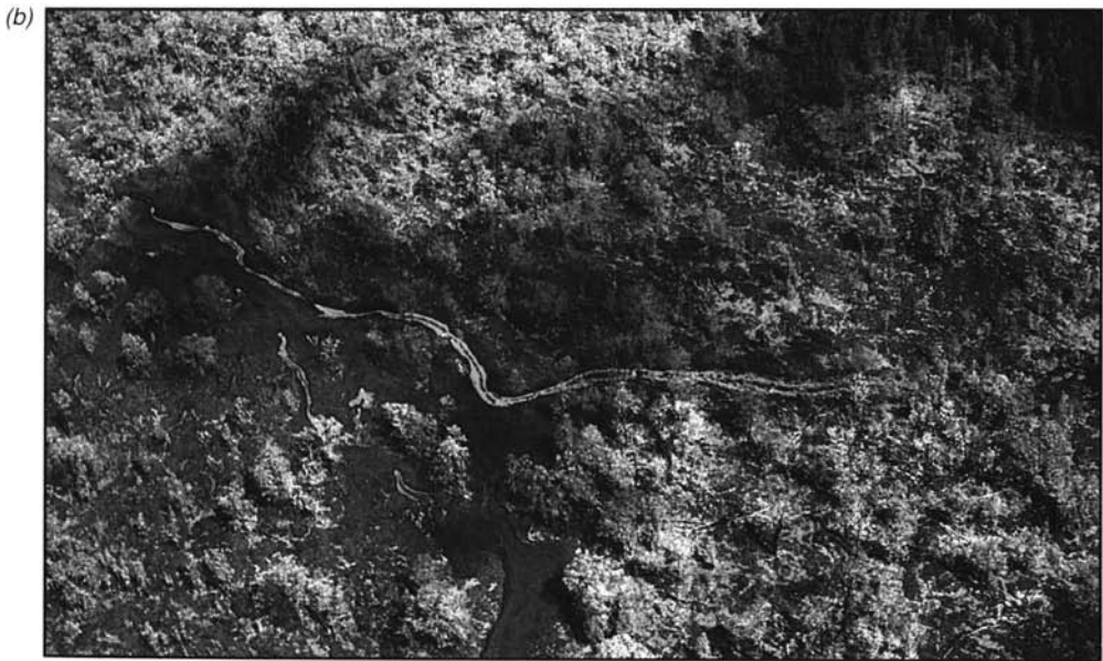
Plate 4 Oblique normal color (a) and color IR (b) aerial photographs showing flowing lava on the face of Kilauea Volcano, HI. The orange tones on the color IR photograph represent IR energy emitted from the flowing lava. The pink tones represent sunlight reflected from the living vegetation. (For major discussion, see Section 2.8.)
