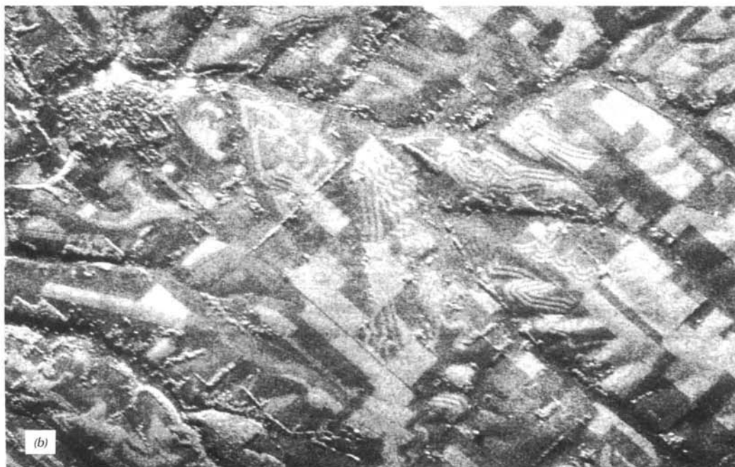
Figure 8.24 SLAR images, southwestern Wisconsin, late summer, X band, synthetic aperture. (a) Prairie du Chien and vicinity. 1: 80,000. (b) Rural area near Prairie du Chien. 1: 50,000. (Courtesy Strategic Air Command and Goodyear Aerospace.)
