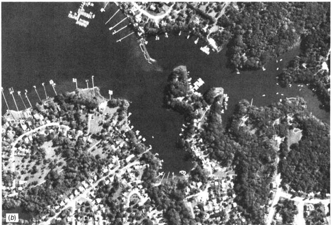
Figure 2.40 Multiband digital camera images, Chesapeake Bay, MD, early October. (a) Blue band, (b) green band, (c) red band, and (d) near IR band. Scale 1 : 9000. (Courtesy Positive Systems, Inc.)
