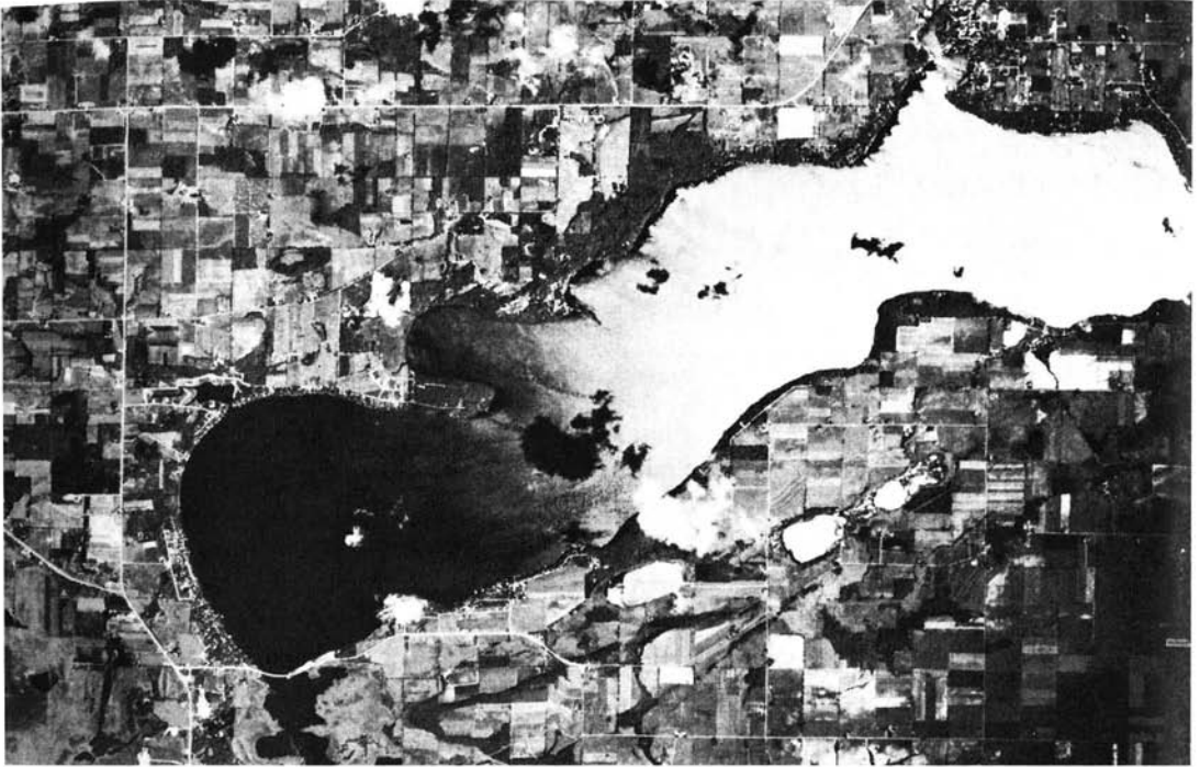
figure 2.8 Aerial photograph containing areas of specular reflection from water bodies. This image is a portion of a summertime photograph taken over Green Lake, Green Lake County, WI. Scale 1 : 95,000. Cloud shadows indicate direction of sunlight at time of exposure. Reproduced from color IR original. (NASA image.)
