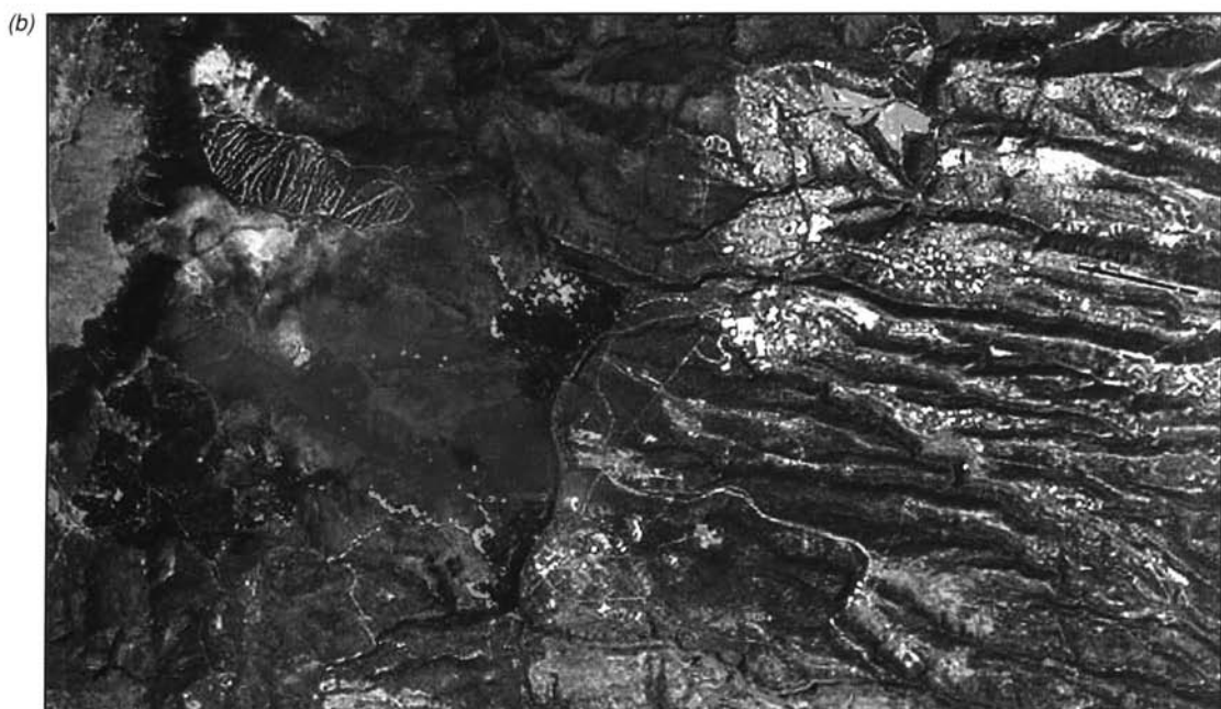
Plate 11 Landsat-7 images showing a wildfire burning near the city of Los Alamos, NM, May 2000. Scale 1:110,000. (a) "Normal color" composite of bands 1, 2, and 3. (b) "False color" composite of bands 2, 4, and 7. In (b), note that the hottest burning areas appear bright red-orange in color, visible because of the strong emitted energy from the fires in the 2.08 to 2.35- \mu\text{m} wavelength sensitivity of band 7. (NASA image.) (For major discussion of these images, see Section 4.15. For major discussion of Landsat-7, see Chapter 6.)
