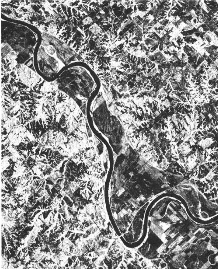
Figure 8.42 SIR-C image, Missouri River near Glasgow, MO. Black and white reproduction of a three-band color composite image (L band HH, L band HV, and L band HH + HV). North is to the bottom of the image. Scale 1: 220,000. (Courtesy NASA/JPL/Caltech.)
