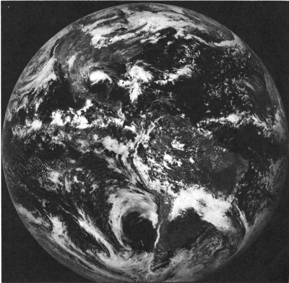
Figure 6.36 GOES-2 visible band (0.55 to 0.7 \mu\text{m} ) image of hemispherical disk including North and South America, early September. A hurricane is clearly discernible in the Gulf of Mexico. (Courtesy NOAA/National Environmental Satellite, Data, and Information Service.)
