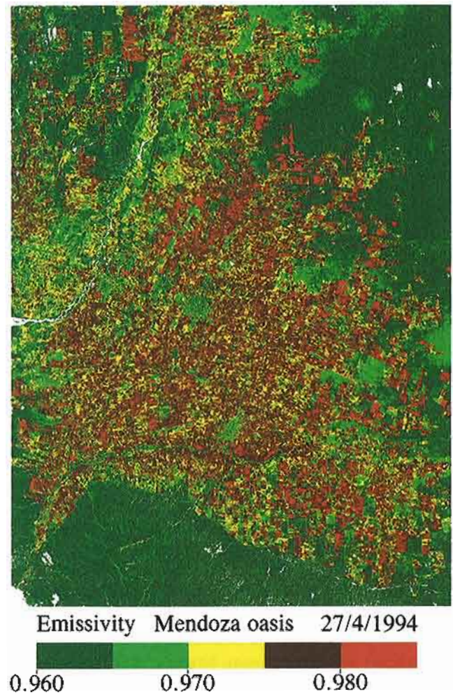
Figure 9. Emissivity map of the Mendoza oasis at Landsat/Thematic Mapper scale. White pixels mark watery surfaces. We can clearly see the contrast between the oasis (in the center, higher emissivities) and the desert (in the surroundings, lower emissivities). In the oasis we can observe the fields well defined and the high density of the crops, which makes the emissivity high in this area.
