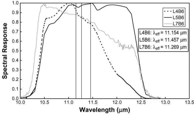
Fig. 1. Spectral responses and effective wavelengths ( $\lambda_{\text{eff}}$ ) for band 6 of Landsat-4 (L4B6), Landsat-5 (L5B6), and Landsat-7 (L7B6) platforms. Vertical lines are the position on the  $x$ -axis of  $\lambda_{\text{eff}}$ .
